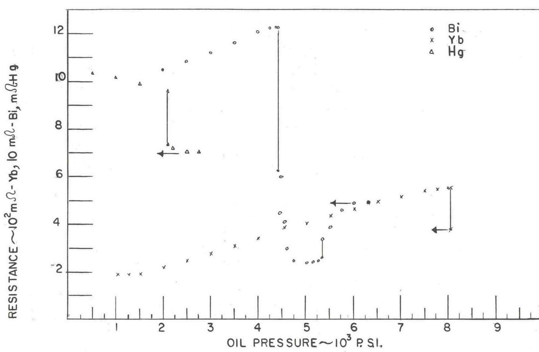
Figure 14. Calibration Phase Transitions for Bi, Hg, and Yb
